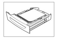
Make sure the paper stack does not exceed the load limit mark.
